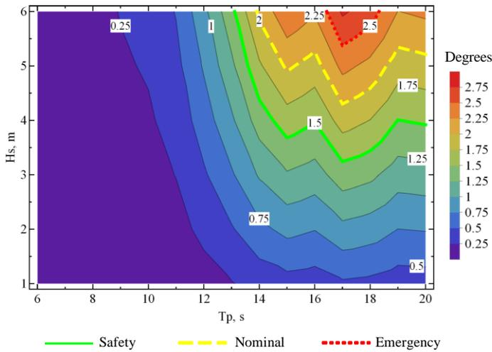
Figure 5. Diagram with limit contours of extreme values for FPSO roll.
