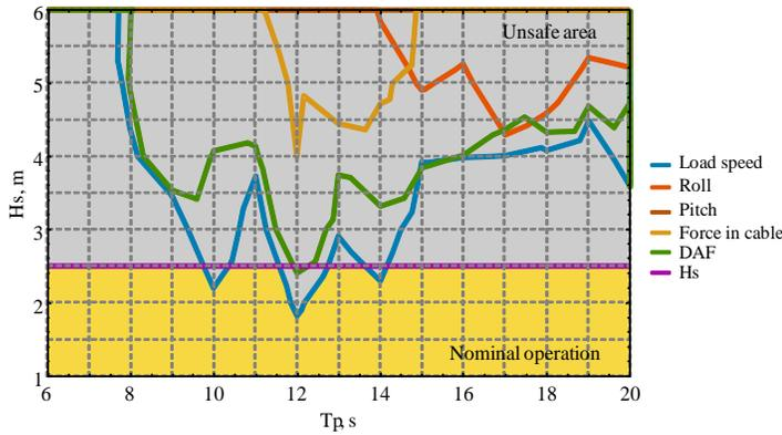
Figure 10. Intermediary operational diagram with limit contours and envelope for nominal operation.
