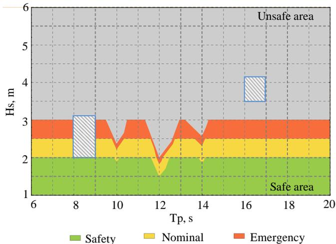
Figure 17. OCOLD including limitation of  $H_s$ , configured to lift personnel, highlighting the necessary area for each application.
