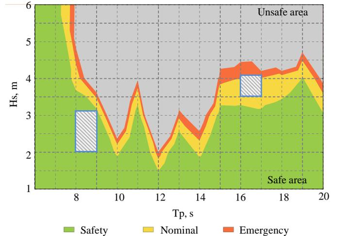
Figure 18. OCOLD excluding  $H_s$  limitation, configured to lift personnel, highlighting the necessary area for each application.
