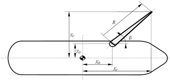
Figure 4. Dimensions and parameters of FPSO [6].
