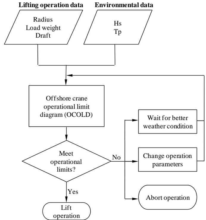
Figure 3. Flowchart for decision-making using the OCOLD.
