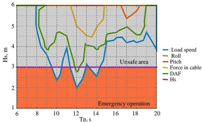
Figure 11. Intermediary operational diagram with limit contours for emergency operation.
