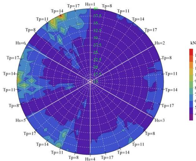
Figure 7. Extreme values for axial load in crane cable in function of Hs, Tp and cable length.
