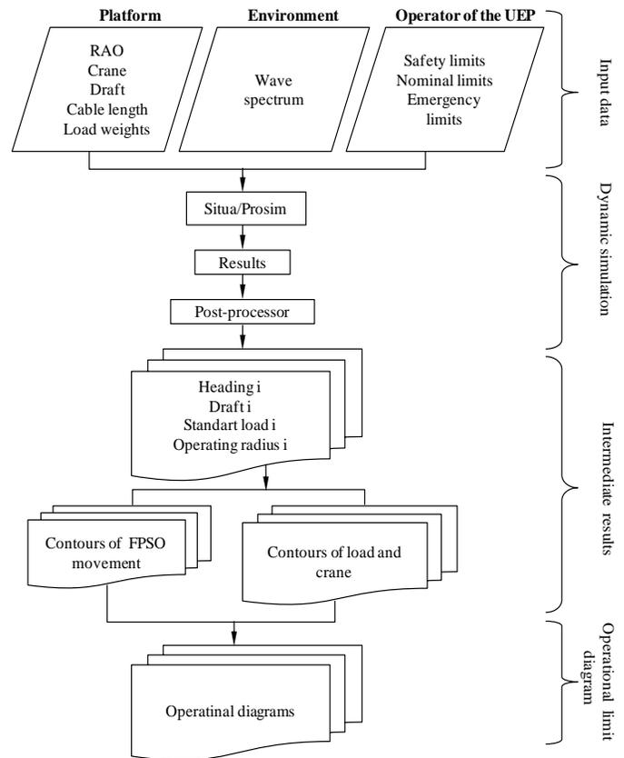
Figure 1. Flowchart for offshore crane operational limit diagram.
