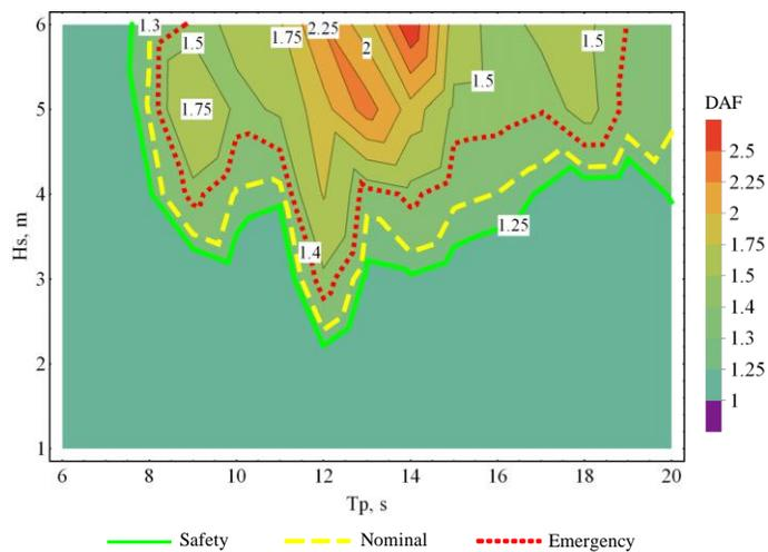
Figure 9. Diagram with limit contours for dynamic amplification factors (DAF) for axial load in crane cable, in function of Hs and Tp.
