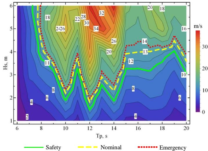
Figure 2. Example of contour plot showing a diagram with contours of extreme values for transport basket speed.
