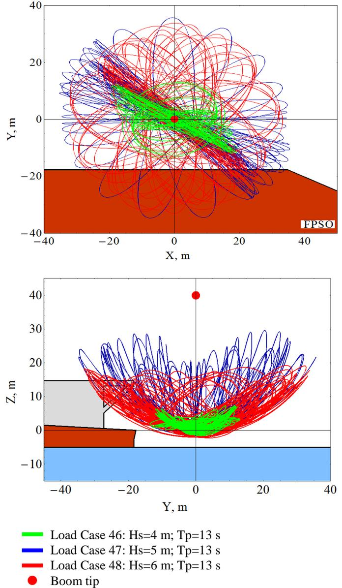
Figure 6. Top view and lateral view for bottom of transport basket path for 3 load cases.
