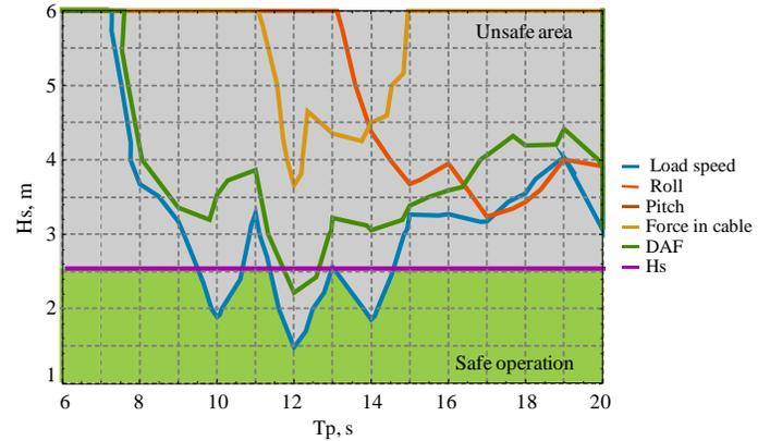
Figure 12. Intermediary operational diagram with limit contours for safety operation.
