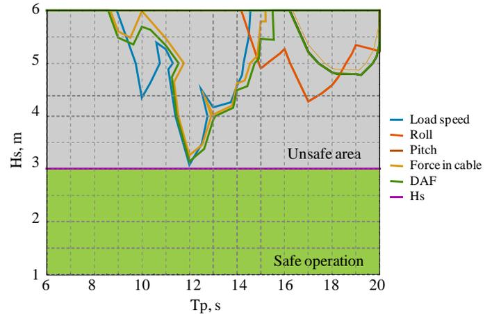
Figure 15. OCOLD including limitation of  $H_s$ , configured to lift general cargo.
