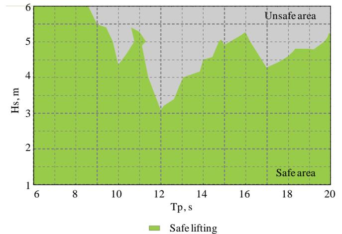
Figure 16. OCOLD excluding limitation of  $H_s$ , configured to lift general cargo.
