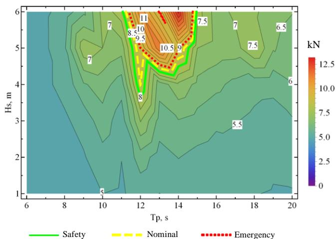
Figure 8. Diagram with limit contours for extreme values for axial load in crane cable, in function of Hs and Tp.
